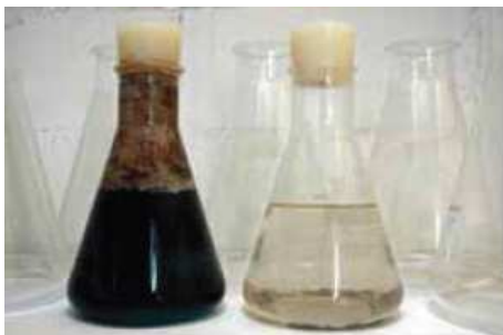
Non- treated & treated effluent samples Sample of heavy oily sludge before and after biological treatment in PETROX™ (pre-filtration). The treated water is subsequently filtered to remove solid matter.
